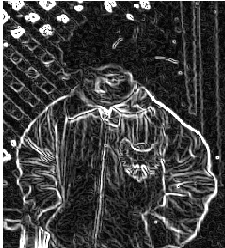
Gradient magnitude, using Sobel masks
